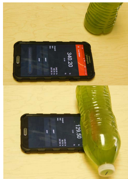
Above: The smartphone app reads the initial amount of ambient light present. Then (bottom) it reads the light passing through the algae culture.
