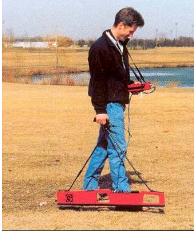
Fig 19. EM38® electrical conductivity meter suspended a few inches above ground during a measurement
