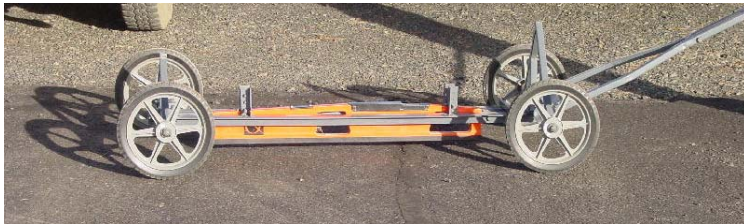
Fig 20. EM38® electrical conductivity meter mounted on a non-metallic cart to leave a few inches above ground. The height of the meter above the soil surface can be adjusted.
