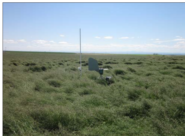
Figure 1. A Burkard volumetric 7-day recording spore trap and weather data logger deployed in a commercial Kentucky bluegrass seed production field (Benton County, WA).
