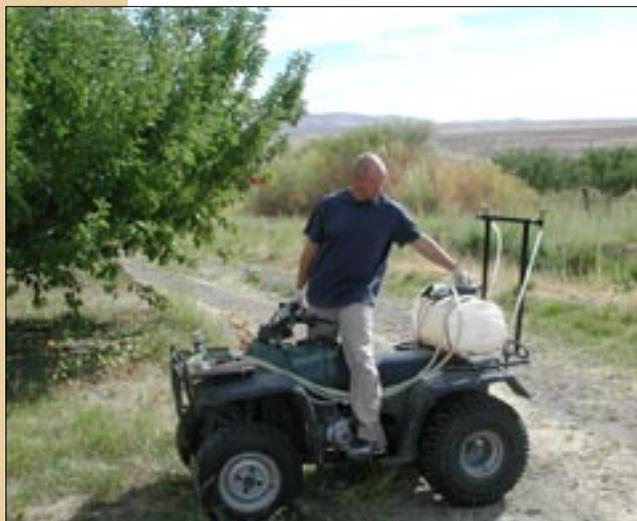
Figure 11a (above).—An all-terrain vehicle is used to apply a microencapsulated formulation of sex pheromone.
