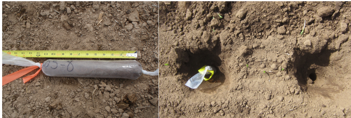
Figure 1. Buried bag before installation (left) and installed into an auger hole before backfilling (right)
