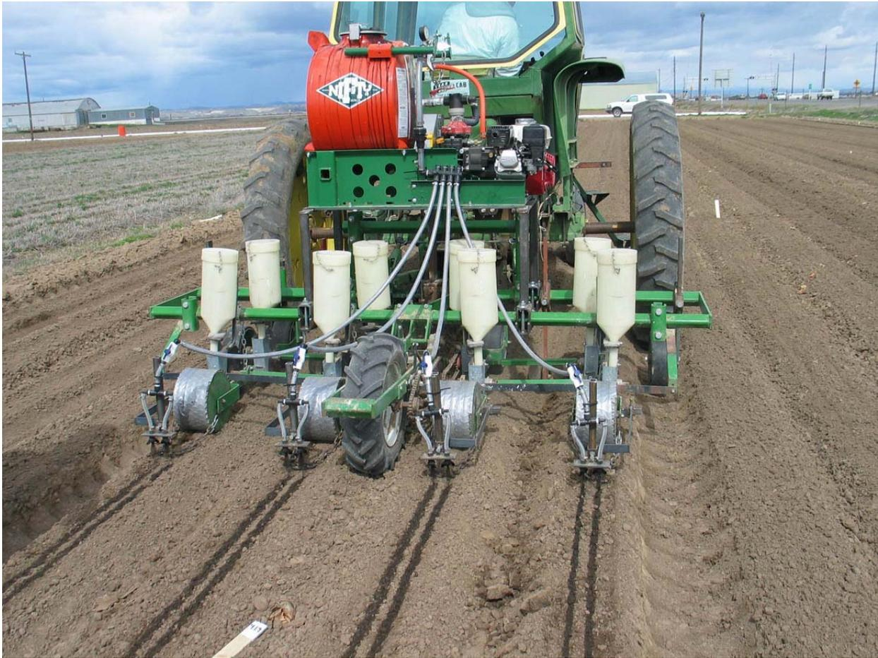
Figure 1. Modified onion planter fitted with a 25-gal Rear's Nifty Tank Series to apply a 1-inch band of charcoal slurry directly over the onion row, Malheur Experiment Station, Ontario, OR, 2009.
