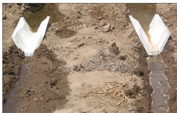
Figure 3. Sediment is reduced in ditches treated with polyacrylamide (left), compared to untreated ditches (right).
