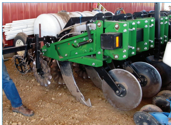
Figure 4. A strip-till unit allows cultivation only within the row zone.
