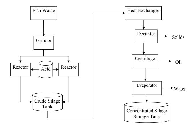
Figure 12 Flow diagram for production of advanced silage.
