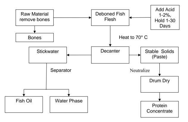
Figure 13 Modified silage process.
