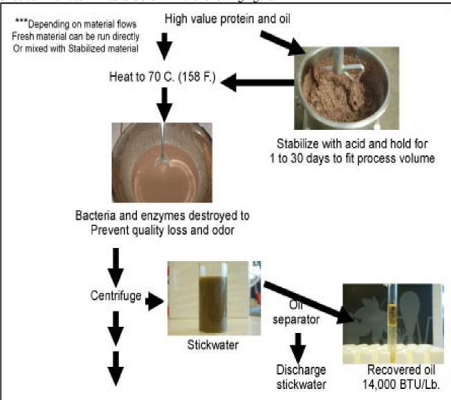
The modified silage process and protein concentrate process envisioned for small to medium sized communities in Alaska is shown in the following figure.
