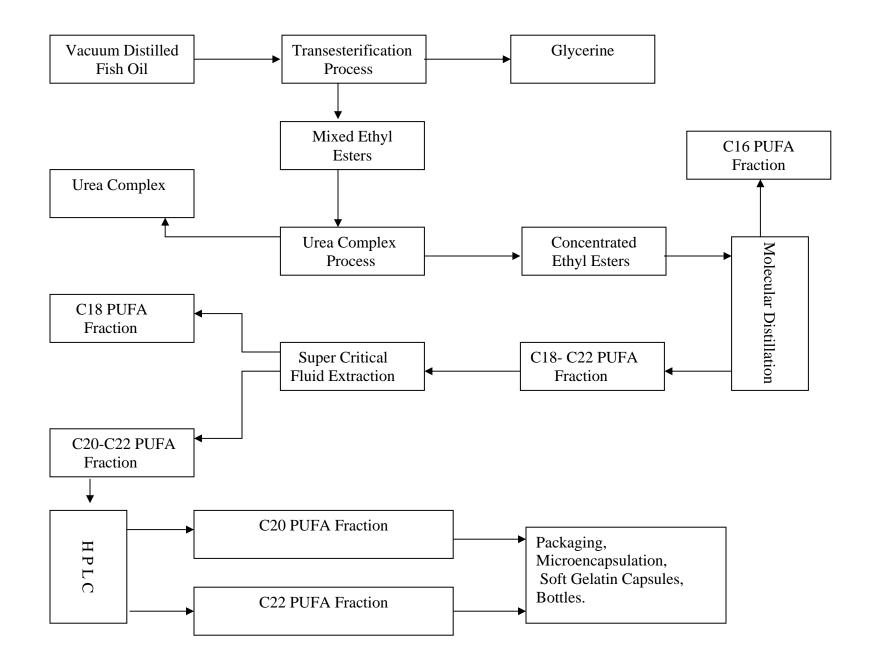
Figure 37 Production of nutraceutical grade fish oil fractions.
