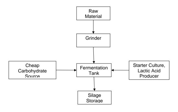
Figure 17 Bacterial fermentation silage process.
