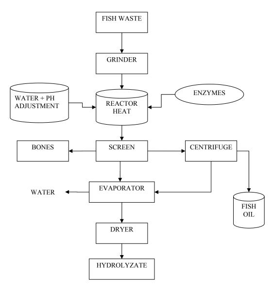
Figure 16 Flow diagram for production of fish protein hydrolyzate.
