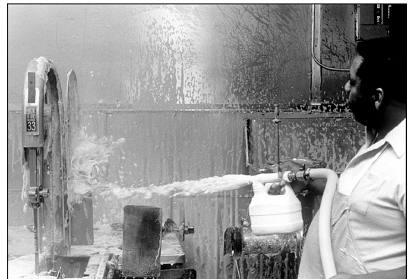
Figure 7. Cleaning with foam. Allow several minutes for detergent action.
