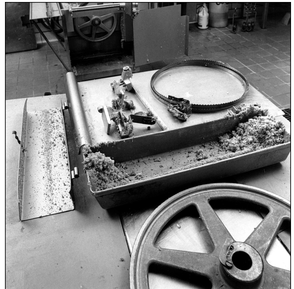
Figure 6. Disassemble equipment for proper cleaning.
