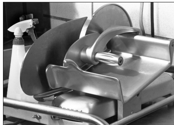
Figure 10. A small pump sprayer may be utilized to sanitize disassembled parts or stationary equipment (such as belts, saws or tables).
